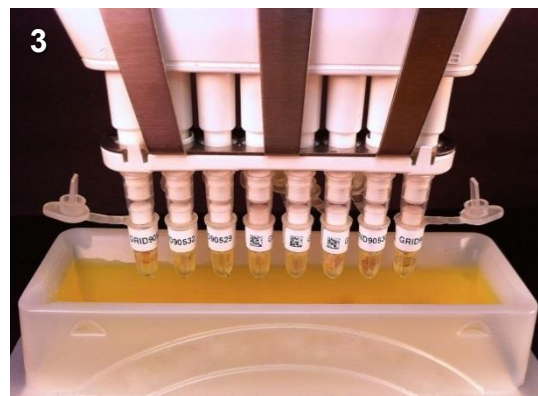
Figure 3: Eight barcode-labeled mPrep/g capsules with grids fitted to an 8-channel pipettor using mPrep/f filter couplers. Capsules contain stain drawn from reagent reservoir.
