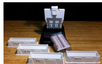
Figure E: Preparation of equipment and supplies for Protocol II. Use a lab stand and clamp to hold the pipettor upright. 8-channel pipettor shown.
