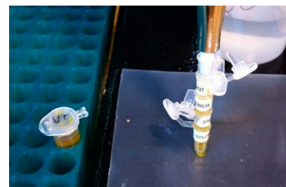
Figure D: Placing the tip of an mPrep/g capsule onto Parafilm.
