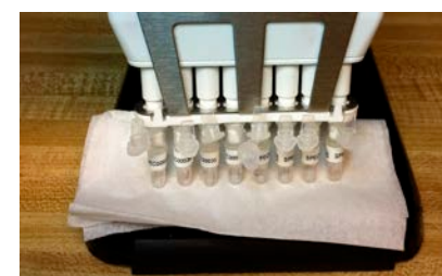
Figure K: Blotting excess fluid from mPrep/g capsules.
