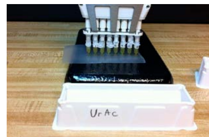
Figure H: Placing capsules on Parafilm during staining.
