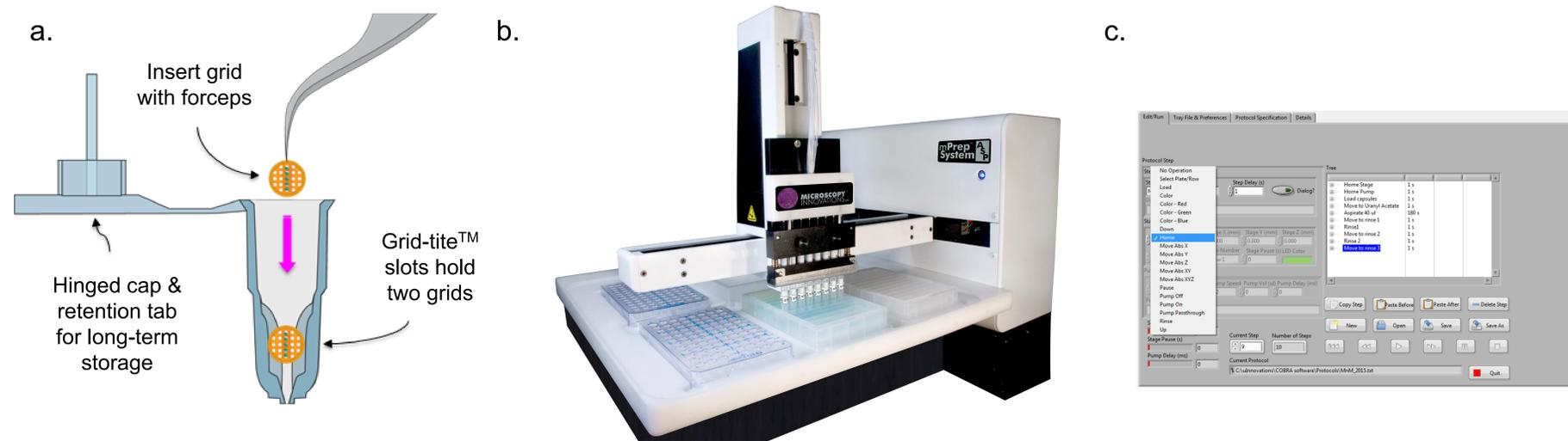
Figure 1. EM grids are inserted into mPrep capsules (a) and are loaded onto the ASP-1000 sample processor (b), which is controlled in easily edited software (c).
