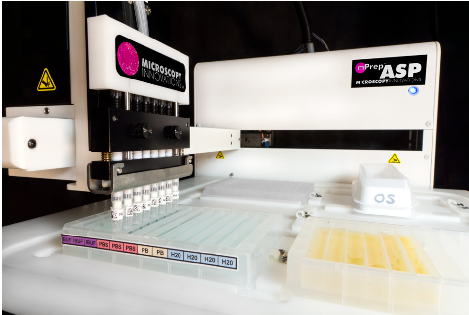
Figure 1: ASP-1000 setup with mPrep/s capsules and reagent plates.
