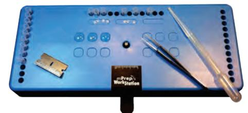
Figure 3: mPrep/s Workstation. The mPrep Workstation was used to orient and entrap the aldehyde-fixed tissue in mPrep/s capsules.
