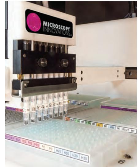
Figure 1: ASP-1000 setup with mPrep/s capsules and reagent plates.
