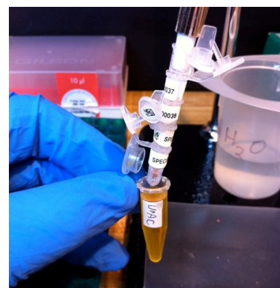
Figure C: Stacking 4 mPrep/g capsules on a single-channel pipettor. Staining with uranyl acetate.
