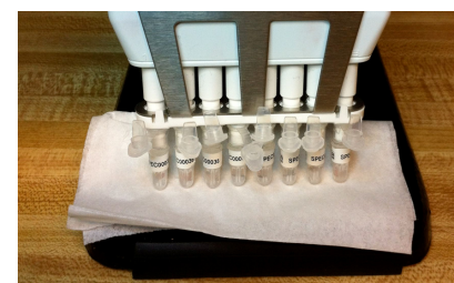
Figure J: Blotting excess fluid from mPrep/g capsules.
