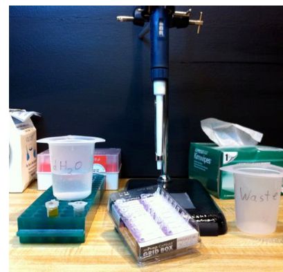
Figure A: Preparation of equipment and supplies for Protocol I. Use a lab stand and clamp to hold the pipettor upright.
