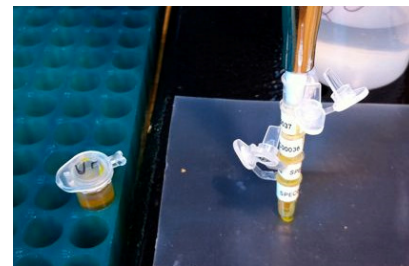
Figure D: Placing the tip of an mPrep/g capsule onto Parafilm.
