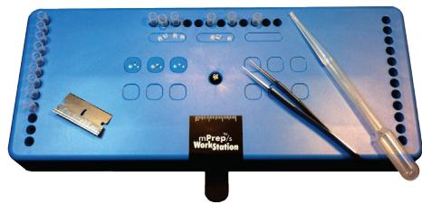
Figure 3: mPrep/s Workstation. The mPrep Workstation was used to orient and entrap the aldehyde-fixed tissue in mPrep/s capsules.
