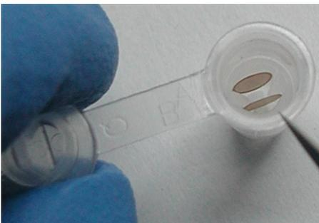
**Figure 3: Capsule loading.** Grids with thin sections or whole-mount specimens are inserted into mPrep/g capsules.
