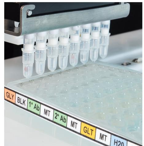
**Figure 2: mPrep/g capsules mounted on ASP-1000 with reagents in microplates on autoprocessor deck.**
