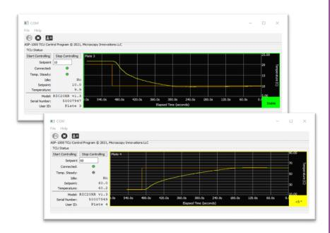
Thermal control dashboard displays temperature in real-time with color coded indications for when temperature is at or approaching its set point.
