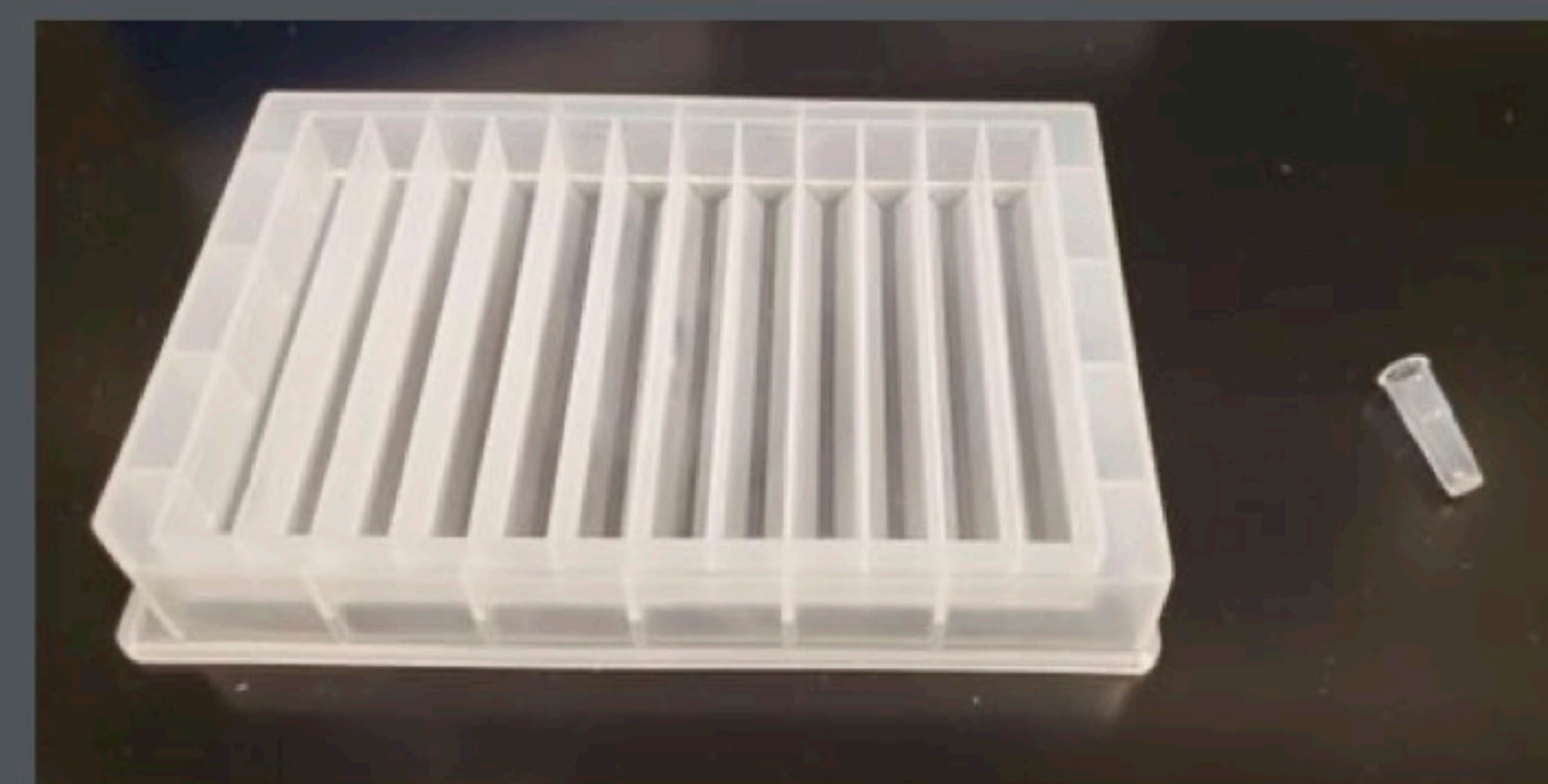
Figure 3. Reagent tray and specimen capsule for the mPrep ASP-1000
